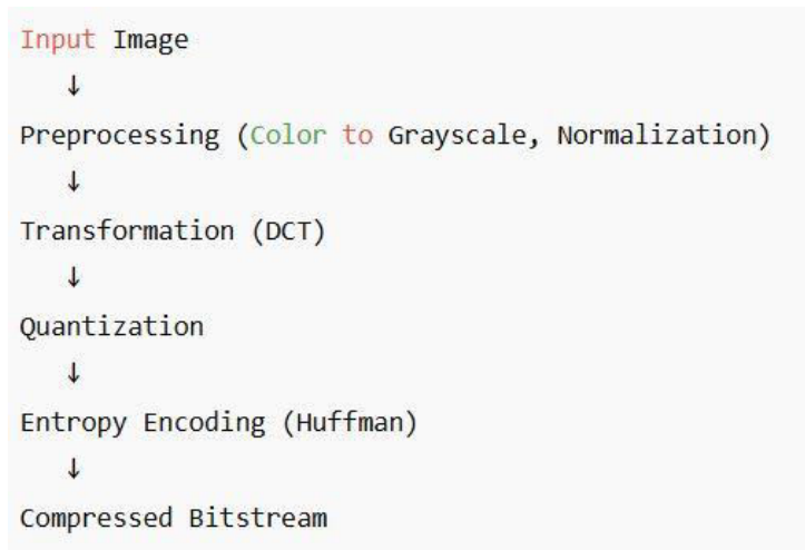
Fig 3.: Method to first converts image data into the frequency domain to remove redundancy, followed by Huffman encoding to compress symbol frequency effectively.
